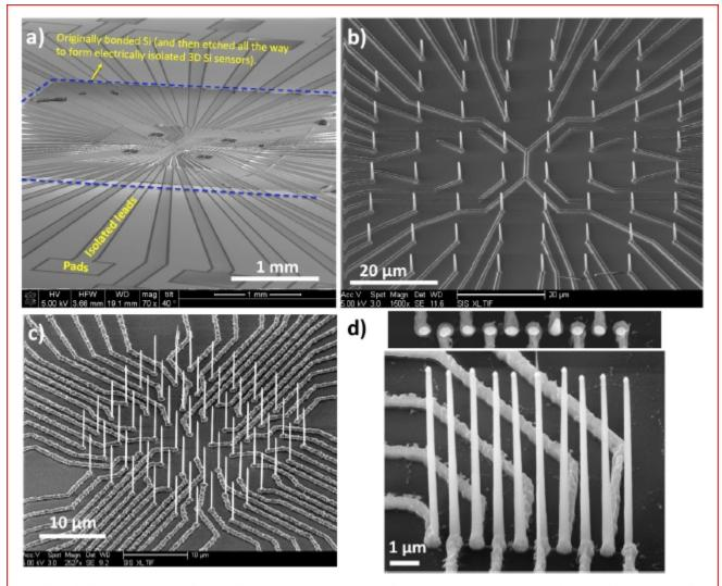
**Figure S3:** SEM images of etched nanowire arrays on sapphire substrate. a) Angle view SEM image of the overall platform after Si nanowire etching. The width of the platform is 1.5 cm. b) SEM image of Si nanowires etched at a pitch of 10μm site-to-site spacing. c) SEM image of Si nanowires etched at a pitch of 4μm site-to-site spacing. d) SEM image of a linear array of Si nanowires etched at a pitch of 750nm site-to-site spacing.
