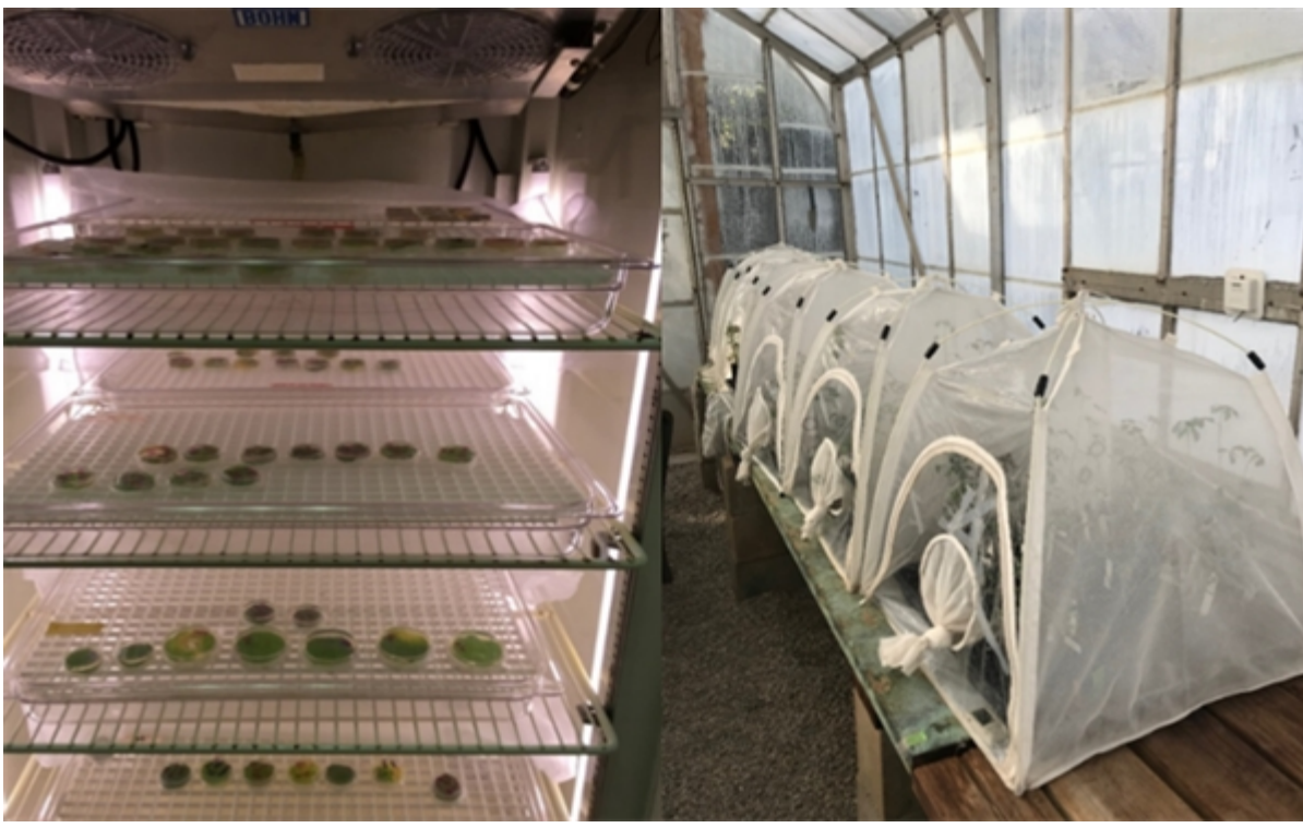
Fig. 2 Each incubator (left) can hold up to 700 experiments/mini-whitefly colonies compared to the bugdorm (right), which houses one colony/experiment per tent. One incubator would replace ~11 biosafety level 2 (BSL2) greenhouses.
