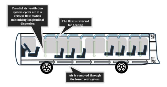
A schematic illustration of the parallel bus cabin air ventilation system - in contrast to current ventilation systems where air travels along the length of the bus and so do air borne pathogens and pollutants.
