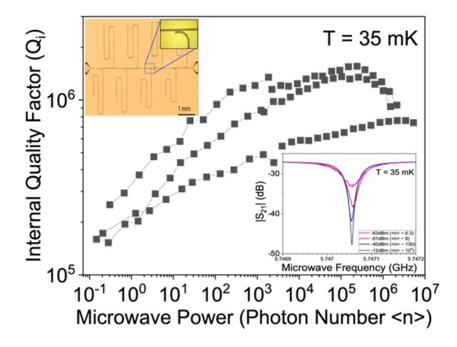
Q-factor for 3 typical quarter wave superconducting resonators
