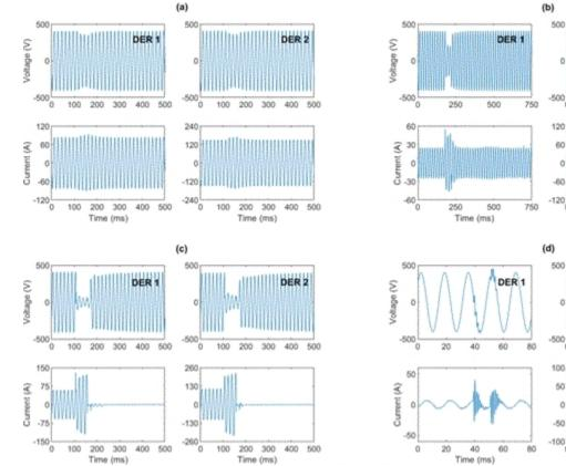
Application of time-synchronized waveform measurements in benchmarking the behavior of DERs on power distribution systems during: (a) a
