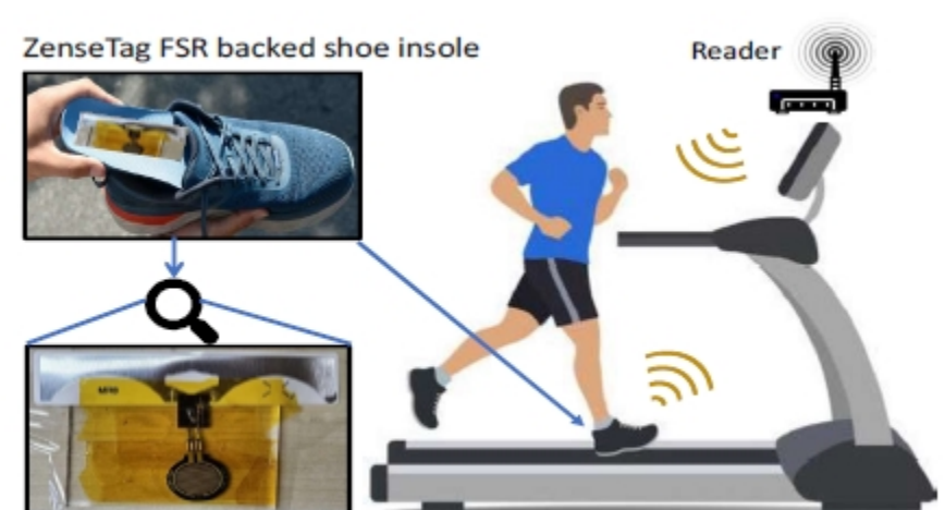
(b) Battery-free wearable shoe-insole based force sensing.
