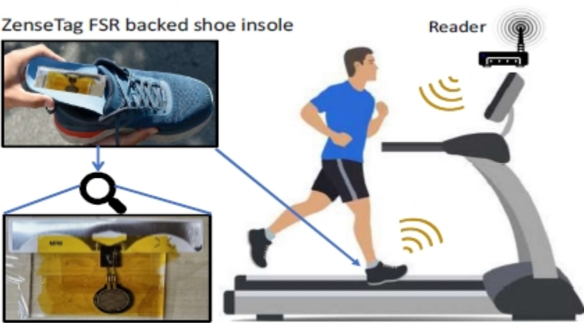
(b) Battery-free wearable shoe-insole based force sensing.
