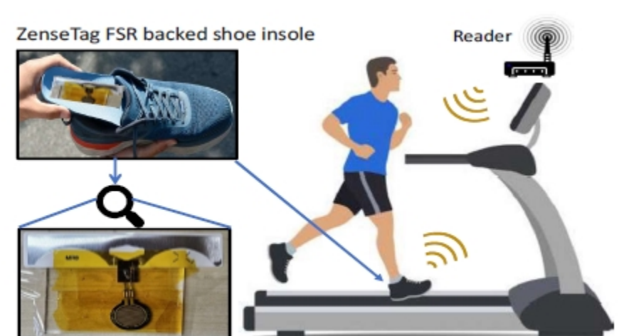
(b) Battery-free wearable shoe-insole based force sensing.
