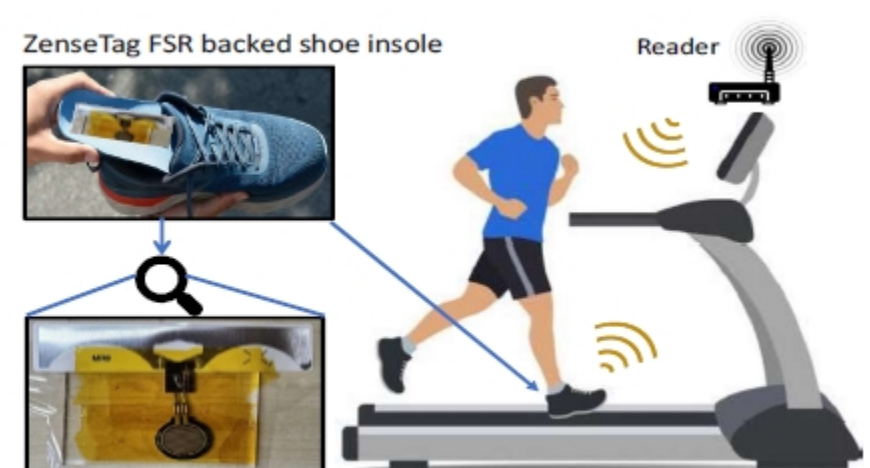
(b) Battery-free wearable shoe-insole based force sensing.
