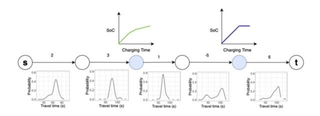
Schematic illuatration of the EV navigation algorithm. The roads have two weights - a travel time distribution (below) and an expected energy depletion or charging (above).
