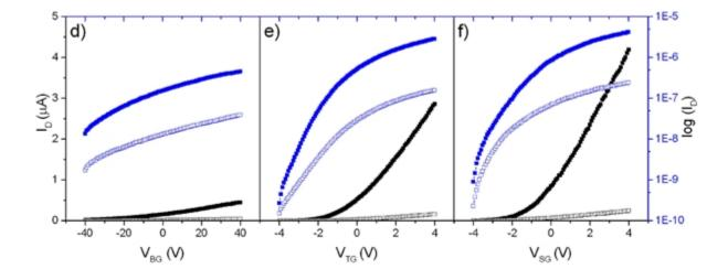
Gate transfer plots (d to f) with the linear axis on the left in black color and the log axis on the right in blue. The curves with filled markers correspond to a  $V_{DS}$  bias of 1V; those with empty markers have  $V_{DS}$  of 100 mV.
