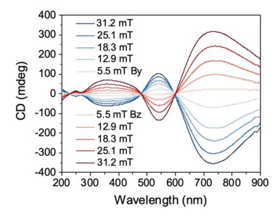
CD spectra of the magnetic/plasmonic hybrid nanorods assembled under magnetic fields with varying direction and strength.
