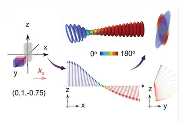
Schematic illustration of the magnetic assembly during chiral dichroism (CD) measurement and simulated helical superstructures assembled from magnetic nanorods under such a chiral magnetic field.
