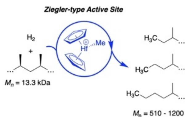
Fig 1: Details the new UCR method to degrade polymers. After 24 h at 200°C under 1 atm H 2 , polypropylene with Ziegler-type catalyst, forms an oil at 78 % yield.
