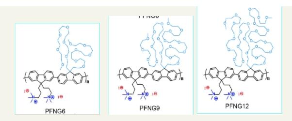
In these exemplary compounds, the backbone is polyfluorene. One fluorene monomer has two ionic (quaternary methylammonium) sidechains with iodide counterions. The second fluorene monomer has oligo(ethyleneglycol sidechains with variable length, corresponding to 6 (PFNG6), 9 (PFNG9) and 12 (PFNG12) ethyleneglycol units.
