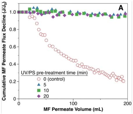
Normalized permeate flux decline as a function of cumulative normalized volume throughput. The brine without the UV/PS pre-treatment has a severe decline in permeate flux due to fouling.
