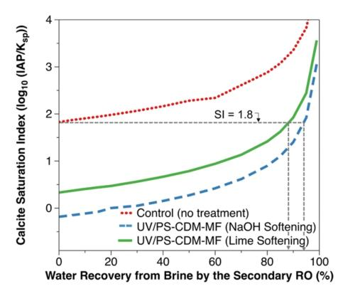
Calcite saturation index revealing the pre-treatment with anti-scalant significantly increases the freshwater recovery.
