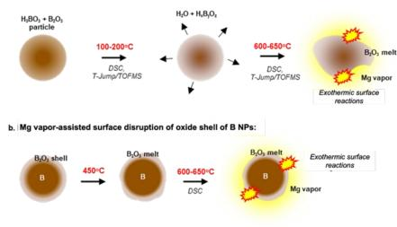
Schematic illustration of the reactivity enhancement of Boron
