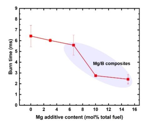
Graph showing the burn characteristics of B/CuO nanoenergetic composites. Mg/B/CuO composites show significant enhancement in burn times and pressurization over B/CuO composites.
