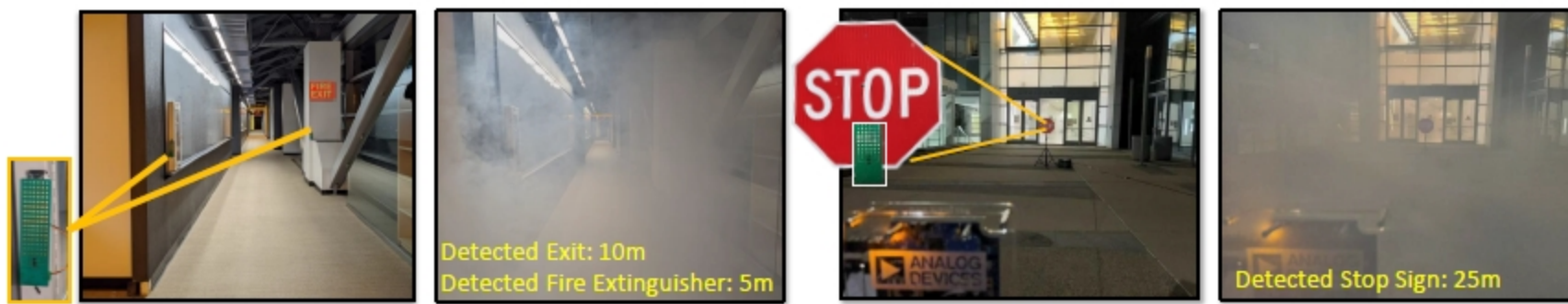
(a) Fire equipment detection through smoke during fire.
