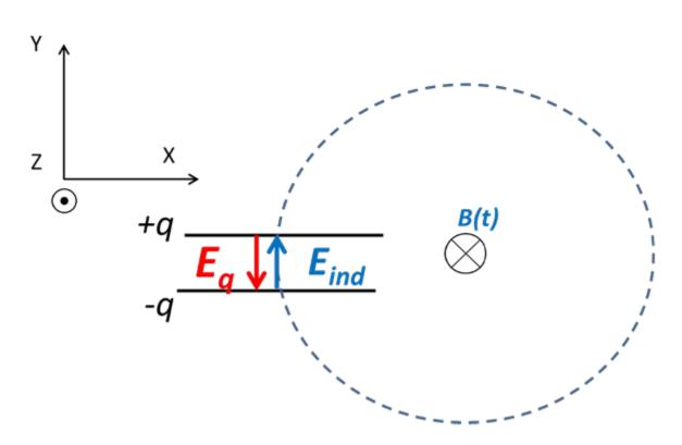
Schematics of a parallel-plate capacitor in a time-varying magnetic field B. The red and the blue arrows show the direction of the electrostatic  $E_{q}$  and the inductive electric field  $E_{ind}$ , respectively. The direction of the inductive field is chosen to compensate the electrostatic
