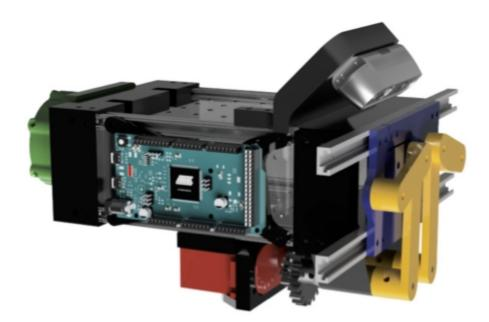
The custom end-effector contains the components necessary to cut a leaf from a tree. The servo motor (red) actuates a double four-bar mechanism (yellow) that closes a set of gates (blue) with a razor blade to cut and capture a leaf. A camera is mounted on the top of the end-effector for perception. A micro-controller is mounted on the arm for controlling the motor. This end-effector can be mounted to a robotic arm using an adaptor plate (green).
