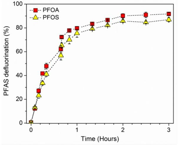
Impact of electron donors on degradation and defluorination of PFOA and PFOS under the irradiation of UV light. [PFOA] or [PFOS] = 25 uM.
