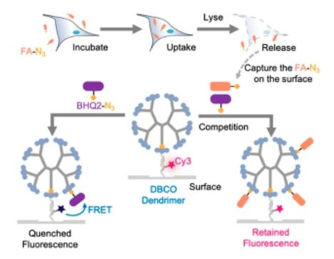
Fig 1: Schematic of the UCR-ISB method for detecting fatty acid uptake from single cells.
