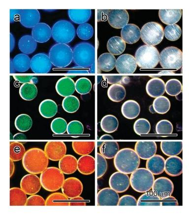
The attached image is optical microscopy images (500x) of magnetochromatic microspheres with diffractions switched between "on" (a, c, e) and "off" (b, d, f) states by using external magnetic fields. These microspheres are prepared using (a, b) 127, (c, d) 154 and (e, f) 197 nm Fe3O4@SiO2 colloids.
