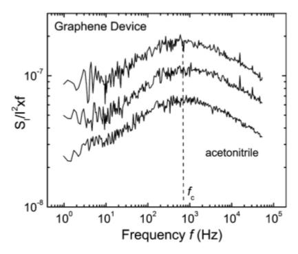
Noise spectral density  $S_1/I^2$  multiplied by frequency f versus frequency f for three different single-layer-graphene transistors exposed to acetonitrile vapor – showing excellent reproducibility.
