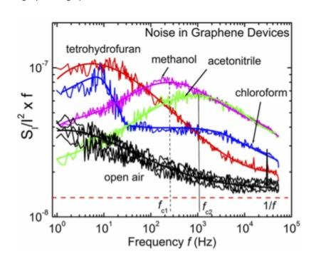
Noise spectral density S<sub>I</sub>/I<sup>2</sup> multiplied by frequency f versus frequency f for the device in open air and under the influence of different vapors.
