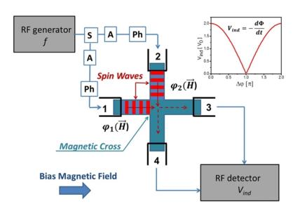
Schematics of the sensing element – a spin wave interferometer built on a magnetic cross junction.
