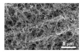
Scanning electron microscopy image of RuO<sub>2</sub> coated NDF.
