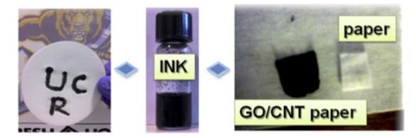
Schematic of non-covalent interaction and preparation of supercapacitor electrodes with GO/SWCNT ink and paper.
