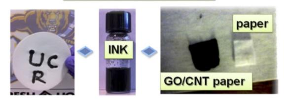
Schematic of non-covalent interaction and preparation of supercapacitor electrodes with GO/SWCNT ink and paper.
