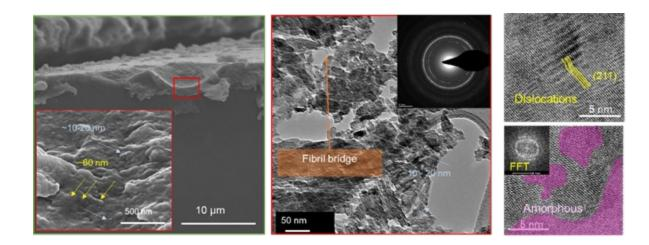
Energy dissipation mechanisms of the bicontinuous particles. Left and middle micrographs show particle breakage and fiber bridging after high
