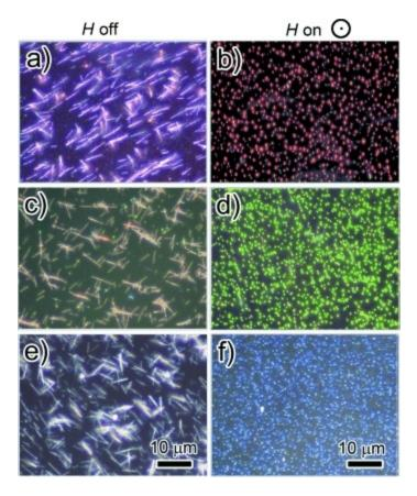
Dark-field optical microscopy images of magnetic photonic chains with different diffraction colors switched between "off" (a, c, e: without magnetic field) and "on" (b, d, f: with vertical magnetic field) states. These photonic chains diffract at different wavelengths because they were prepared using Fe3O4 CNCs of different average sizes: a, b) 182 nm, c, d) 160 nm, e, f) 113 nm. All images are at the same scale.
