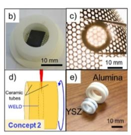
(a) Schematic illustration of concept 1 above; (b) picture of a sample electronic payload (an integrated chip) placed inside a ceramic tube; (c) picture of a successfully welded assembly of concept 1 - the background pattern (pitch 3.5mm is visible through a transparent ceramic cap); (d) schematic of concept 2 for welding simple ceramic geometries; and, (e) picture of a successfully welded assembly of alumina and ytria-stabilized zirconia (YSZ).
