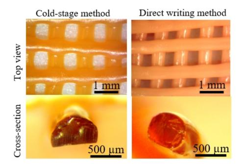
Fig 1: Optical micrographs of top view and cross-section of HyA hydrogels printed using cold-stage method and direct writing method. Hydrogels printed using direct writing method showed
