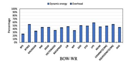
Fig 1: shows the dynamic energy normalized to the baseline GPU for BOW-WR across fifteen different benchmarks. The small segments on top of each bar represent the overheads of the structures added by the idea. Dynamic energy savings in Fig 1 are due to the reduced number of accesses to the register file as BOW-WR shields the RF from unnecessary read and write operations.
