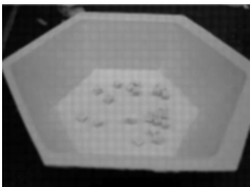
Fig. 2 Dried cubes of TiO 2 mixed with PVA dispersing agent
