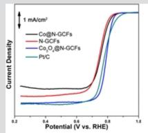
Fig. 2 Linear sweep voltametry curves shows that the graphitic nanofibers doped with metal ions have higher current densities than commercial platinum on carbon (Pt/C).
