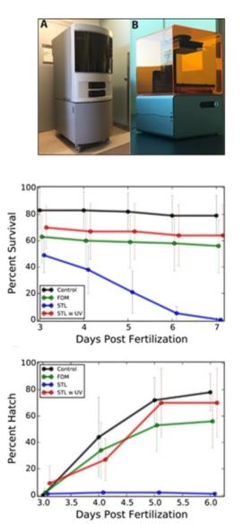
Top image: A is 3D FDM printer. B is a 3D STL printer. The middle graph shows the survival rates of exposed zebrafish embryos when compared to control unexposed embryos. The bottom graph shows the hatching rates of exposed zebrafish embryos when compared to control unexposed embryos. The zebrafish embryos are exposed to 3D-printed parts from a FDM and a STL printer. The STL printed parts when exposed to UV are less toxic when compared to the STL printed parts without UV treatment.
