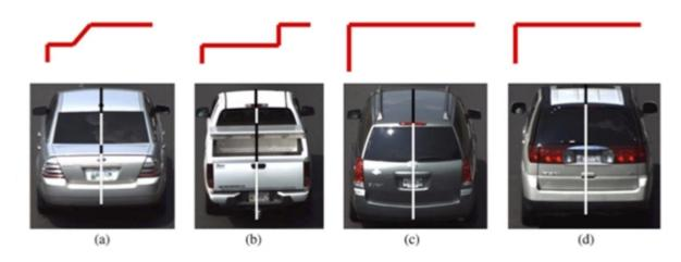
The orange lines at the top show the canonical structures for different vehicles. Bottom pictures show the rear views of corresponding passenger vehicles (a) Sedan, (b) Pickup truck, (c) Minivan, and (d) SUV
