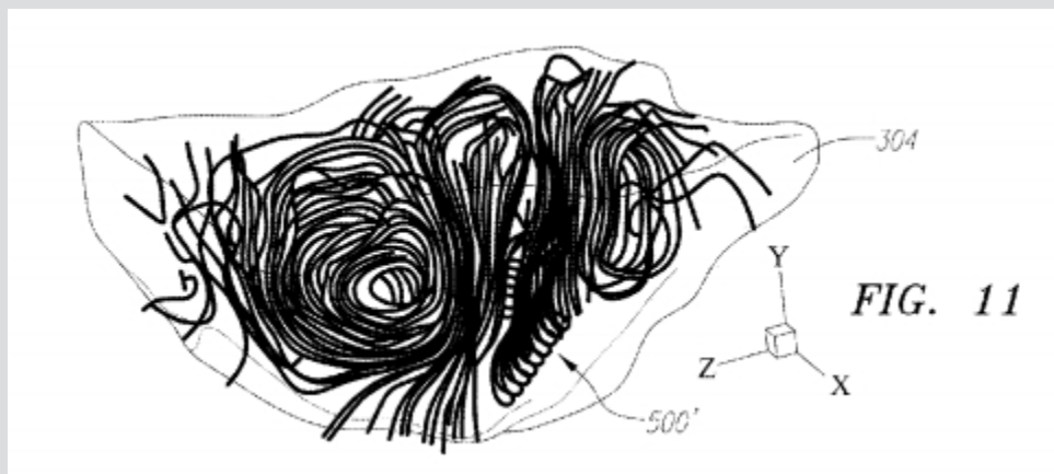
Figure 11. The 3D divergence-free interpolated velocity field inside the right ventricle model is shown during early diastole. The streamlines illustrate the jet and the vortex around it.
