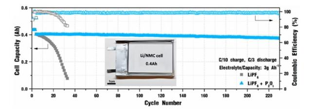
Cycling performance of 0.4 Ah Li||NMC622 pouch cell (50 µm Li anode and 3 mAh/cm<sup>2</sup> cathode areal capacity) in lean electrolyte (electrolyte to capacity ratio = 3 g per Ah) at C/10 charging and C/3 discharging.
