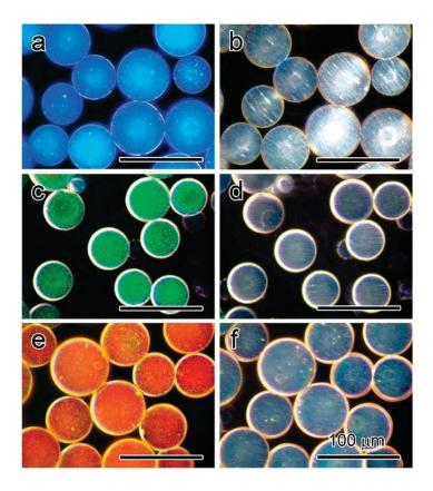
The attached image is optical microscopy images (500x) of magnetochromatic microspheres with diffractions switched between "on" (a, c, e) and "off" (b, d, f) states by using external magnetic fields. These microspheres are prepared using (a, b) 127, (c, d) 154 and (e, f) 197 nm Fe3O4@SiO2 colloids.
