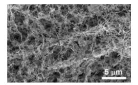
Scanning electron microscopy image of RuO<sub>2</sub> coated NDF.
