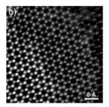
High-angle, annular dark-field scanning, Transmission Electron Microscopy image showing tri-, bi- and monolayer MoS<sub>2</sub> (from left to right).
