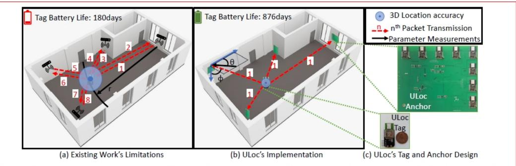
Fig. 1. ULoc: Comparing the traditional UWB localization system to ULoc, showing (a) Low-battery life (180 days) and high latency (8 packet exchanges) (b) High batter life (876 days) and low latency (1 packet exchange) (c) ULoc's custom localization anchor and tag boards, where tag is placed next to a penny, measures only 1.6 × 3.7 cm.
