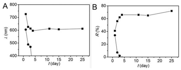
Change in (A) peak position and (B) intensity of the diffraction of aqueous solutions containing Fe3O4@p-SiO2 (square) and polyacrylate-capped Fe3O4 particles (circle) assembled under fixed external magnetic fields after the particles are stored in water for various times. For Fe3O4@p-SiO2 particles the field strength is -131G and the field gradient 77.5 G/cm, while for the polyacrylate-capped Fe3O4 particles, the field strength is -162 G and the field gradient is 82.5 G/cm
