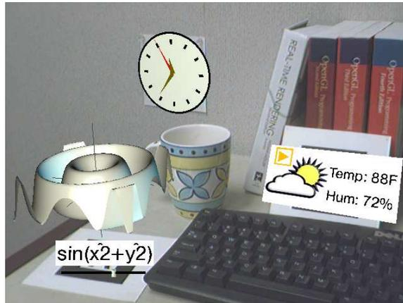
**Figure 2.1:** A typical ARWin desktop, with clock, weather station and graphing calculator applications attached to markers in the environment.
