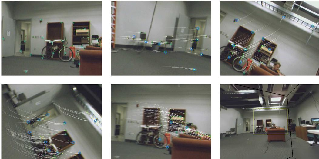
**Figure 3.24:** Snapshots of the feature tracking for hand-held camera motion over five minutes. *Left to right, top to bottom:* (a) Initial feature set. (b,c,d,e) Tracking maintained through various speeds and orientations, with landmark reacquisition. (f) The resulting partial environment map shows the quality of the tracking.
