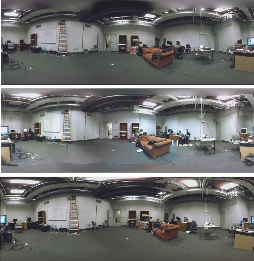
**Figure 3.25:** Cylindrical projections of acquired environment maps. *Top to bottom:* (a) Using a tripod. (b) With automatic exposure and white balance enabled, creating visible discontinuities due to intensity and hue differences. (c) Carefully constructed with a hand-held camera in approximately 3 minutes. Small translations result in errors.
