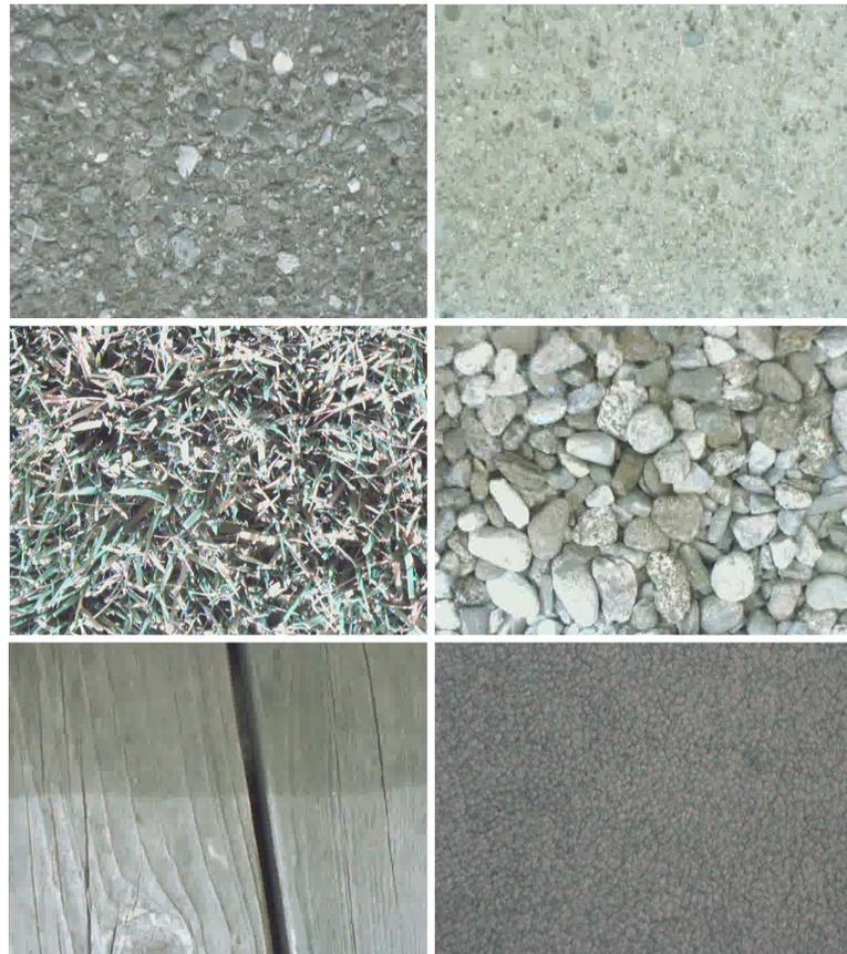
**Figure 3.7:** Different types of terrain with example slip rates. *Left to right, top to bottom:* asphalt (65%), concrete (80%), grass (20%), gravel (32%), wood (24%), carpet (48%). Slip rates depend on speed, jitter, lighting and debris, in addition to texture contrast.
