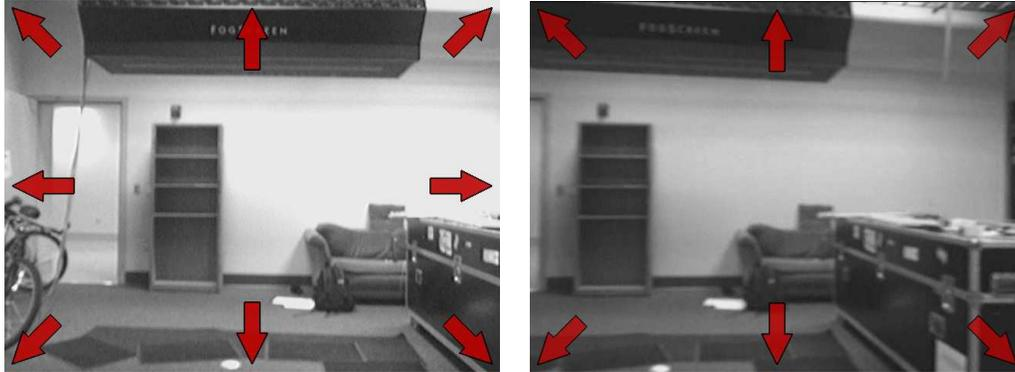
**Figure 3.17:** On-screen feedback in the form of arrows around the video image direct the user’s acquisition. *Left to right:* (a) Before panning the camera, all directions need to be acquired still. (b) After the camera has completed a circular path, the left and right arrows are gone.
