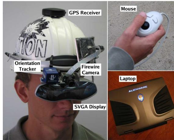
**Figure 3.1:** The ARagorn base wearable system hardware. An Alienware Area-51 m5500 laptop (worn in a backpack), an SVGA Sony Glasstron PLM-S700E display, a Point Grey Firefly firewire camera, An InterSense InertiaCube2 orientation tracker, a Garmin GPS 18 receiver, and an ErgoTouch RocketMouse.
