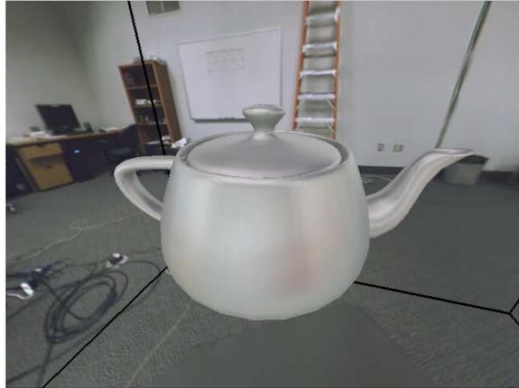
**Figure 3.21:** Virtual geometry shaded using the acquired environment map from Figure 3.25(a). The environment map is filtered first to create the appearance of a silver material with a glossy finish. The teapot is superimposed over the acquired environment map.
