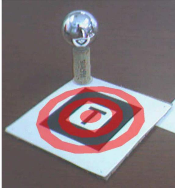
**Figure 2.5:** An ARToolkit marker with a light probe attached. The bullseye shows the marker has been recognized.
