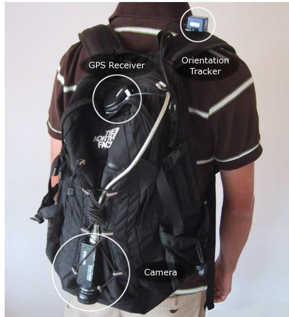
**Figure 3.4:** The modified ARagorn wearable setup for GroundCam tracking. We use a Unibrain Fire-i 400 camera, an InterSense InertiaCube2 orientation tracker, and a Garmin GPS 18 receiver.
